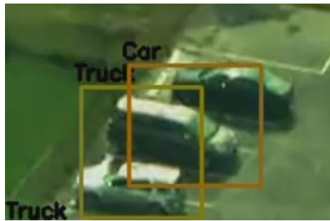
Figure 4: The bounding box surround two vehicles at a time. For an object counting task perspective, this algorithm performs poorly, however, for a detection task, this algorithm performs correctly.
